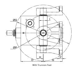
Trunnion mounts provide a pivot point at the gearbox of the screw jack.
