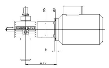
Mount an electric motor to the C-Series screw jack with the extensive range of motor adaptors designed to be used in conjunction with a flexible jaw coupling that connects the motor drive shaft to the screw jacks worm shaft.
