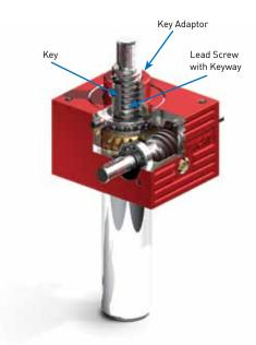
The Anti-Rotation feature for translating screw jacks stops the lead screw from rotating without the need for end fixing. This is done by keying the lead screw. However the keyway in the screw will cause slightly greater than normal wear on the internal threads of the worm gear.
